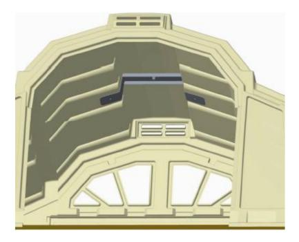
Looking from inside the hutch, drill the center hole in roof measuring 26.50" from back inside roof edge. Then, drill the other 2 holes using a 9/16 drill.
