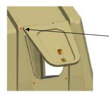
**Step 3: Fasten Star Washer:** From inside of hutch, place star washer (pushnut) over straight end of access door rod.
