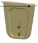
**Step 3: Fasten Star Washer:** From inside of hutch, place star washer (pushnut) over straight end of access door rod.
