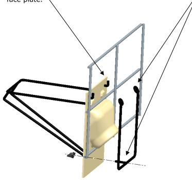
**Step 2: Assemble to Fence:** Align face plate to opening in fence. Insert bottle holder wires through fence, into u-shaped wire support bracket holes. Threaded stud at bottom of u-shaped wire support bracket should be inserted through the lower hole on the face plate.
