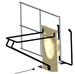
**Step 3: Fasten to Fence:** Tighten wing nut onto stud at base of u-shaped wire support bracket.
