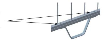
**Step 5: Connect Latch to Frame:** Using the short bolts included in the hardware kit, mount latch plate to inside of front frame. ,
