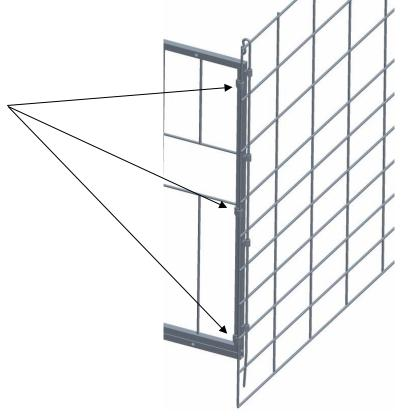
**Step 2: Secure Fence Panels:** Using the provided side panel pin (2), guide pin through fence and frame connectors.
