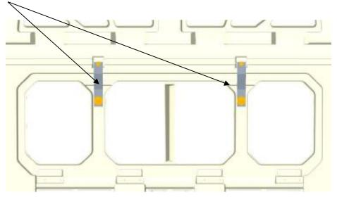
**Step 2:** Remove the inside nut and washer from CH-9225 Latch that locks the bedding door.
