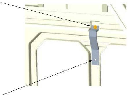
**Step 4:** Using a 5/16" dia drill bit, drill a hole through the plastic using the hole in the Reinforcement Bracket as guide.
