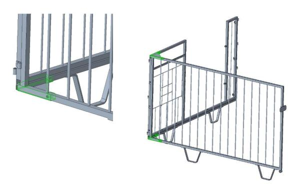
**Step 4:** Connect the Center Front to the opposite side of the front frame of the previous step with 1-1/2'' bolts
