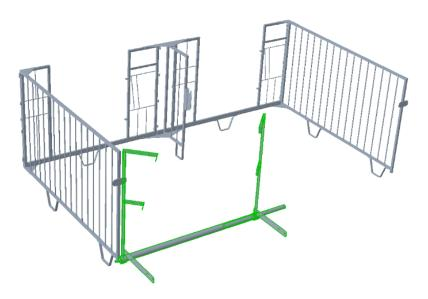
**Step 10:** Slide CT-4008 Center Flip up over the end of the 1<sup>st</sup> pipe.
