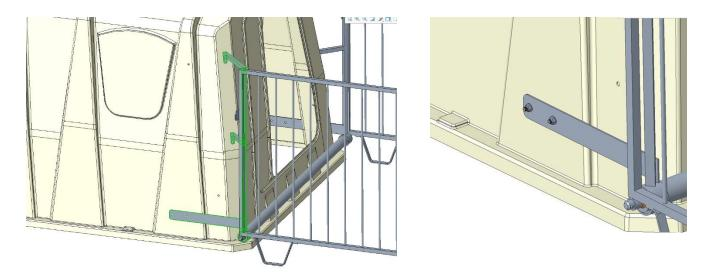
**Step 14: Connect Latch to Frame:** Using 1-1/4" length bolt, attach gate latch to front frame.
