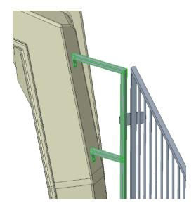
Step 11: Also, mark the hutch through the 2 holes on the lower support bar of the hutch
