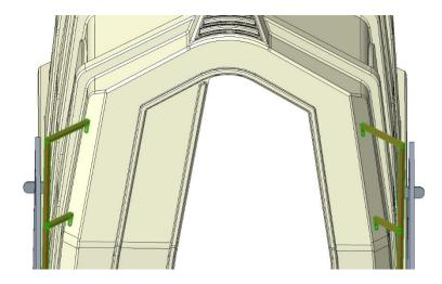
**Step 10:** Using a marking device, mark the hutch through the holes on the tabs of the hutch connection pieces.
