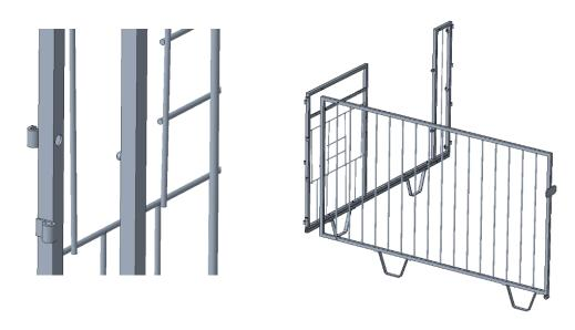
**Step 3: Secure Front Frame to Side Panels:** Attach upper and lower corners with corner brackets and 1-1/2" bolts.
