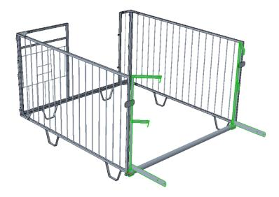
**Step 6:** Insert pipe into bottom back of side panels.
