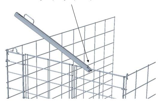
**Step 9:** Locate the center pairing panel (panel with loops on both ends). Align the end with the smaller loops with the loops that are overlapping behind the center front connector. Insert side panel pin through all the loops.
