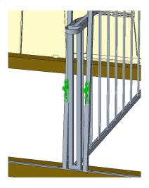
**Step 6: Hang gate:** Start by guiding top hinge on gate through the top hole on frame. Once hinge is in place, follow with the bottom hinge.
