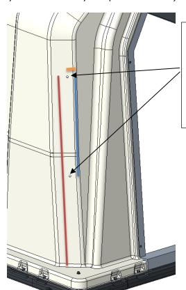
Mark and Drill top 3/8" dia. hole: 34.5" up from plastic base – RED LINE and 1.25" in from plastic face – ORANGE LINE
