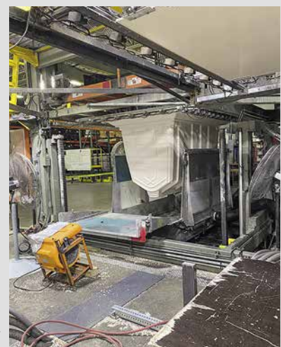
▷ Heated to 165 °C, the plastic sheet is sucked up by a vacuum and formed around a metal structure.
